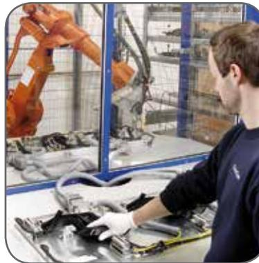
Foaming of lamp holders using an automated robot cell
