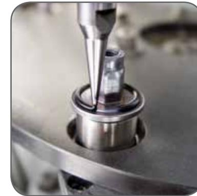
Automatic foaming of threaded bushings in a 3 seconds cycle time
