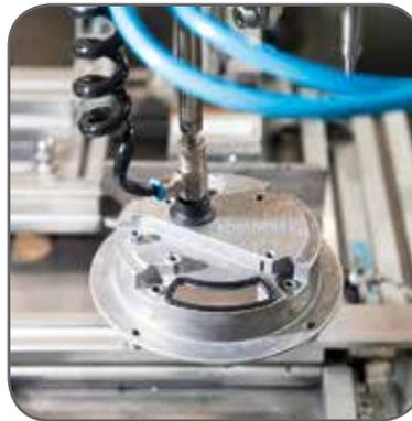
Automatic foaming of covers in a 7 seconds cycle time
