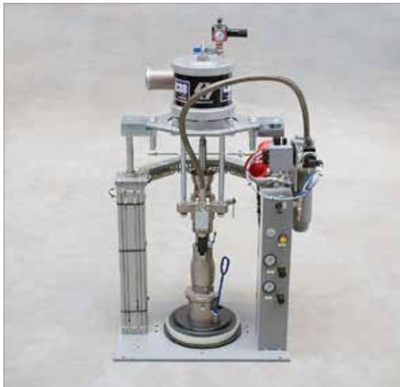
Barrel pump for receiving 20 kg material drum containers
